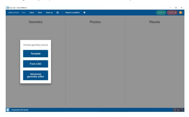
**Template automatically defines the non-critical parts of the simulation setup** and offers new users a **preset simulation physical and geometrical values**, so you only need to change the parameters that are already there.
