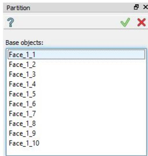
**IMPORTANT:** Partition and Groups are vital for simulation setup with CENOS, because mesh creation as well as physics and boundary condition definitions are based on groups created in this part.
