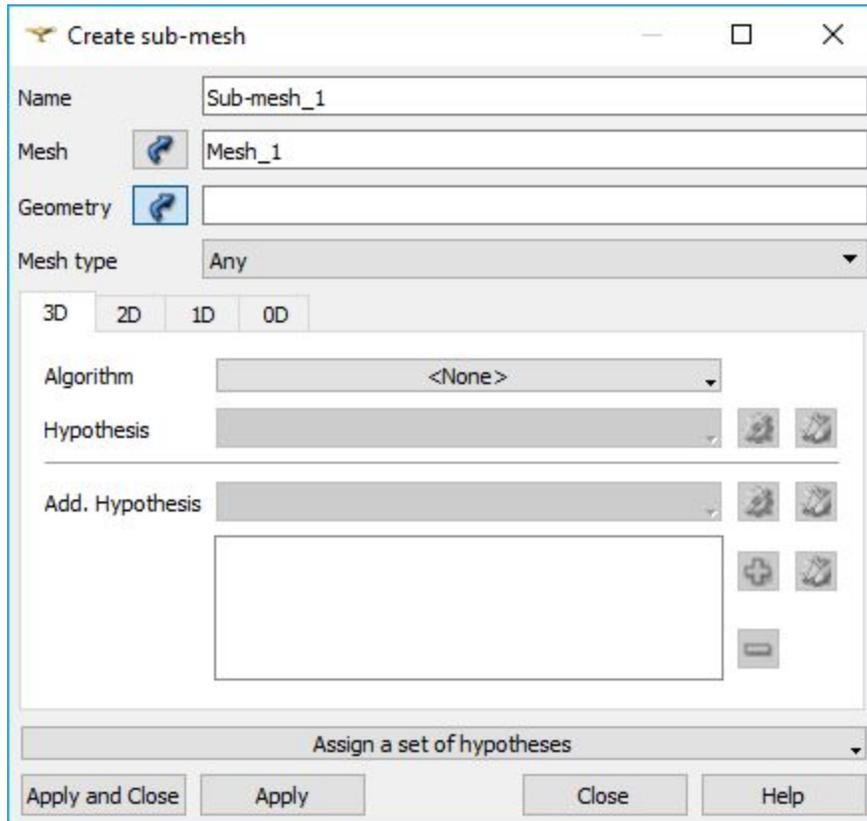
Choose workpiece group from the Partition\_1 dropdown menu as Geometry. From the Assign a set of hypothesis dropdown menu choose 2D: Automatic Triangulation. In the Hypothesis Construction window enter 2 for Max Length.
