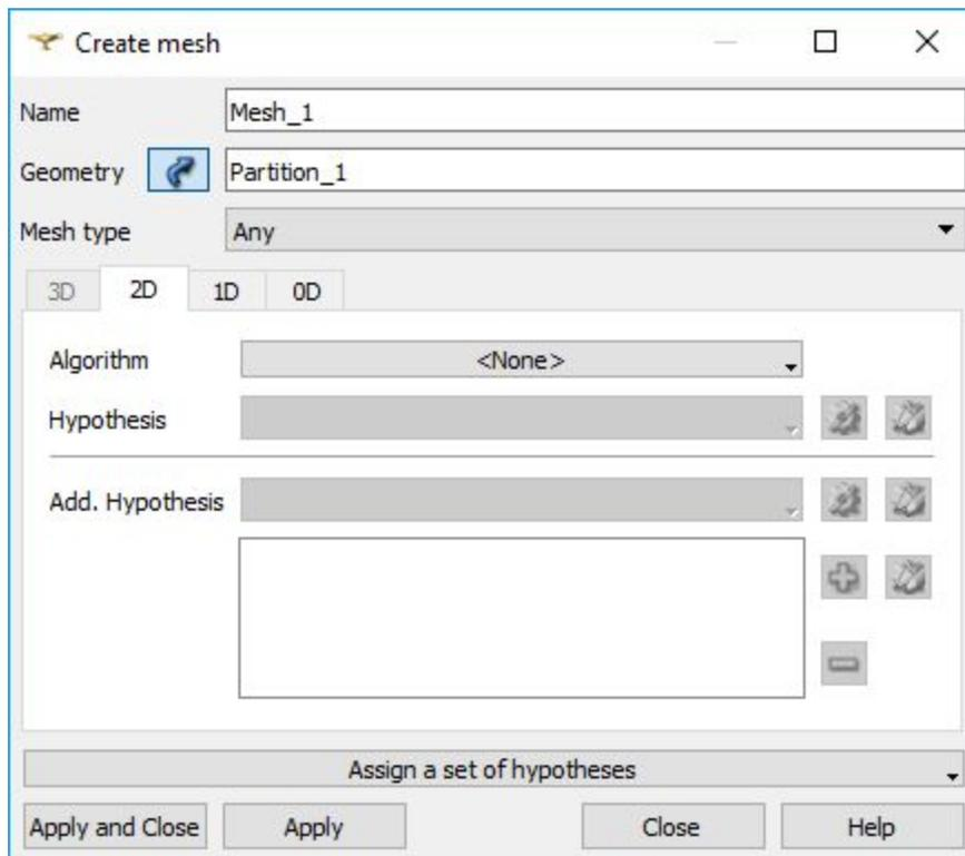
From the Assign a set of hypothesis dropdown menu select 2D: Automatic Triangulation - leave the Max Length value default and click Apply and Close.
